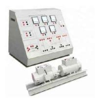
5.2 The training system should have motor & generator on a common rail & should be directly coupled with flexible coupling. The trainer should be provided with control panel and measurement unit. The training setup be supplied with BS10 safety terminals in compliance with IS302-1/IEC60335-1, tested from NABL accredited Lab and Control Panel consist of high grade FRP material for better safety and in compliance with IS302-1/IEC60335-1, tested from NABL accredited Lab.
