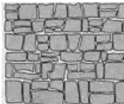
Fig.1.6: Coursed Rubble Masonry
