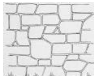
Fig.1.9: Uncoursed Rubble Masonry
