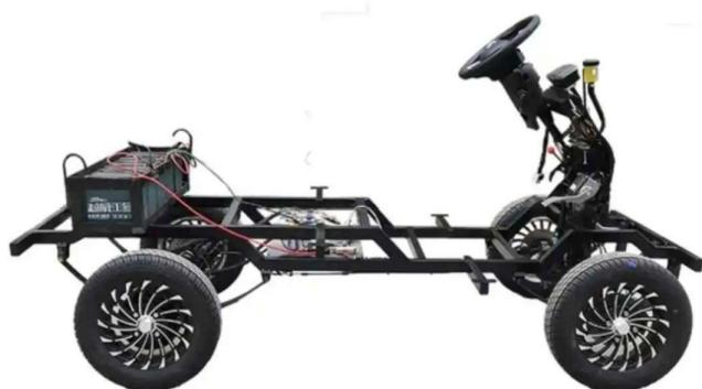
83.2 The Mini Commercial Vehicle chassis structure will be fitted with Front suspension system with Disc brake system, and rear suspension system with Drum brake system, steering system complete, the chassis structure will also be assembled with EV rear axle and EV motor
