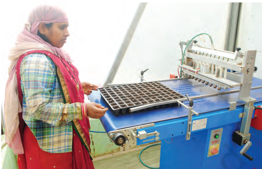
Fig. 2.8: Seed sowing by machine in plug-trays
